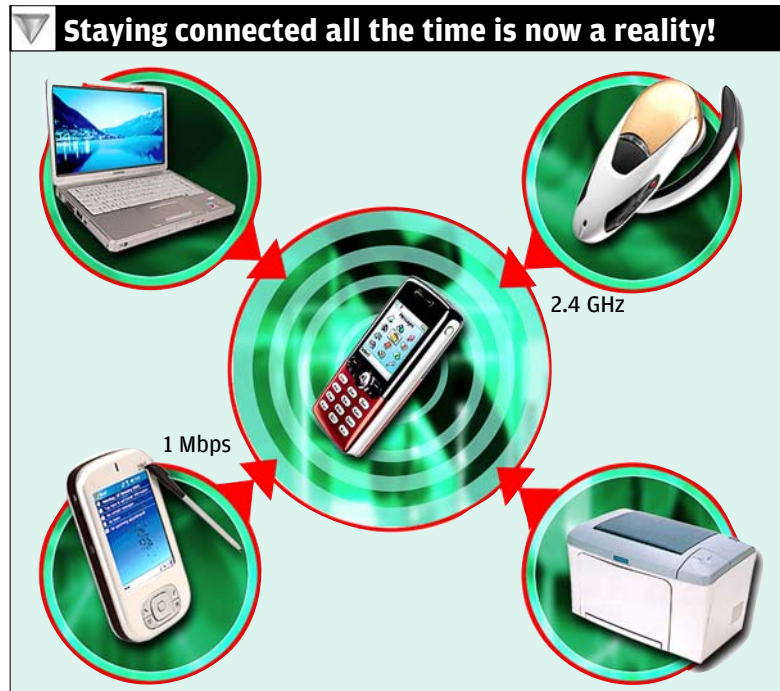
Using Bluetooth, you can achieve data transfer speeds of 1 Mbps between your devices
