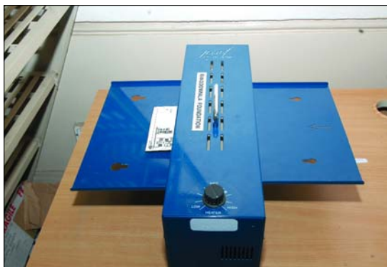
Picture In A Flash or PIAF is used to print tactile graphics
